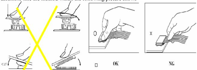
Precaution for soldering to the LCM
